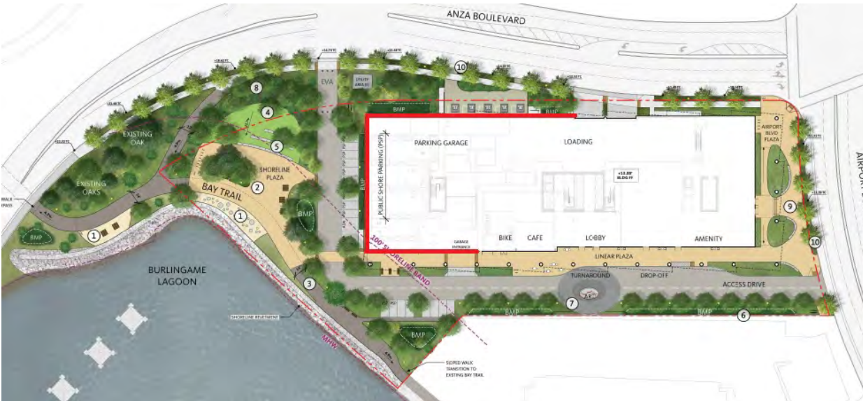
Figure 3. Illustrative site plan. Areas of heightened collision risk with the lower 60 feet of the building are identified in red.
